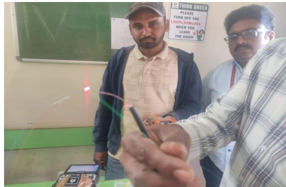
Verification of Output at fiber end after coupling
